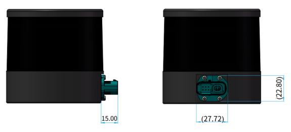
Figure 2.4 Connector Dimensions (Unit: mm)
