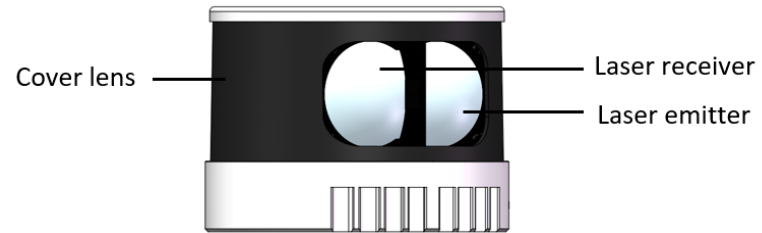
Figure 1. Partial cross-sectional diagram
